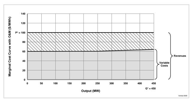
Figure 2.6: Identification of Revenues and Variable Costs by Load Period
