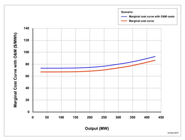
Figure 2.4: Marginal Variable Cost Curve
