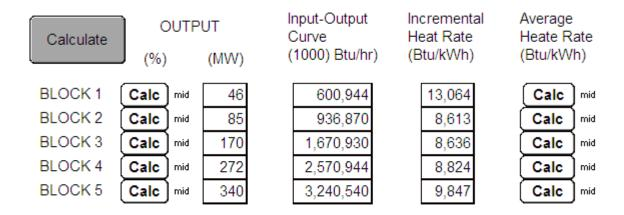
Figure 6.5: Input Screen for Blocks
