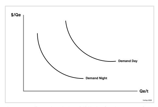
Figure 3.1: Illustration of Diurnal Shifts in Electricity Demand
