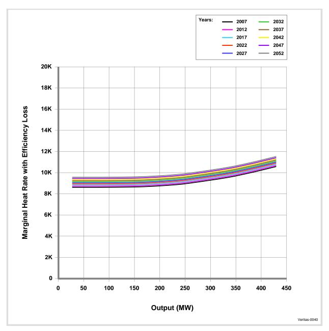
Figure 2.5: Marginal Heat Rate Curve Efficiency Decay
