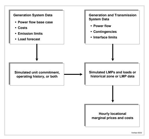
Figure 5.1: Location-Specific Price and Unit-Specific Operation Forecasting Process
